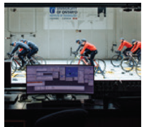
Rigorous testing of its new Merino apparel was undertaken by PEARL iZUMi at the ACE Climate Wind Tunnel in Ontario, Canada.
